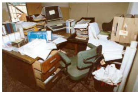
view inside simulated office enclosure before test
