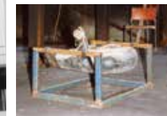
60 litres of petrol in a plastic tank placed inside test structure
