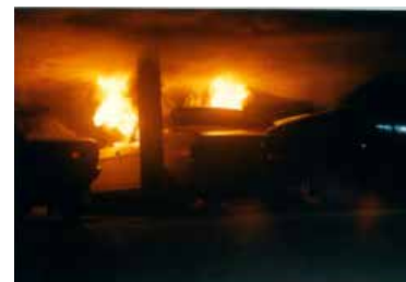
During the fire test view inside test structure showing test vehicle alight
