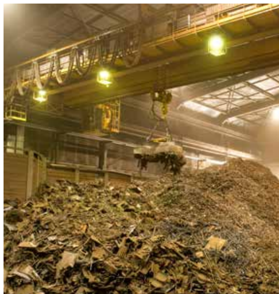
InfraBuild collects and processes scrap steel for use in the manufacture of new steel in its EAFs.
