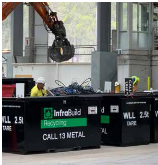
InfraBuild collects and processes scrap steel for use in the manufacture of new steel in its EAFs.
